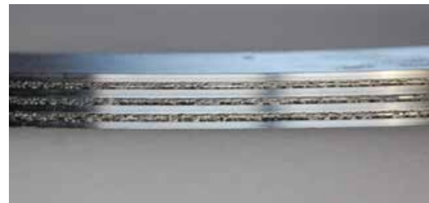
Graphite / inconel lamination for very aggressive chemicals
