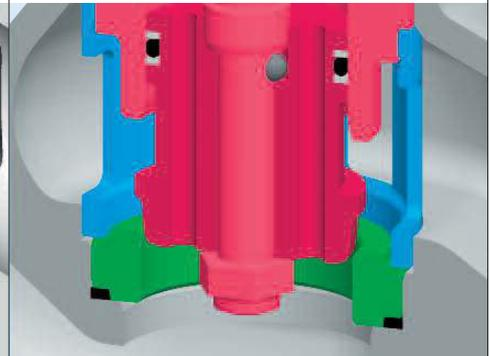
**Pressure-balanced valve plug**
