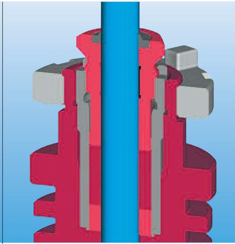
**Cooling fins for high temperatures**
