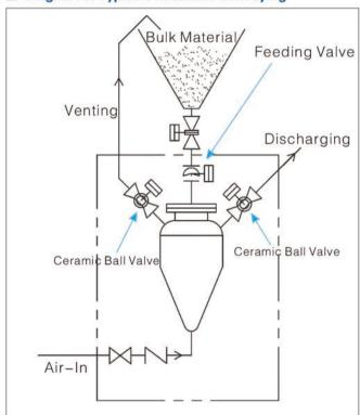
Note: This is a typical pneumatic conveying unit, and other similar systems are also applicable.
